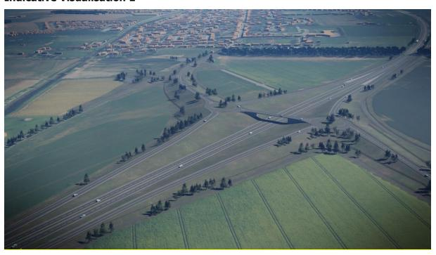
The A90/A937 Laurencekirk Junction Improvement Scheme comprises a new grade-separated junction located at the existing atgrade south junction into Laurencekirk from the A90. The scheme design is shown in **NTS Figure 1.**
