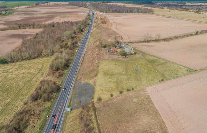
The design of the new dual carriageway required a substantial volume of earth to be removed at this location to accommodate the new A9 southbound
