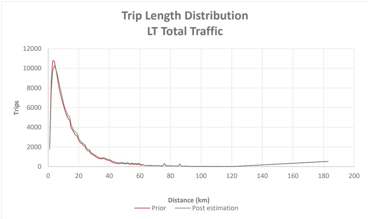
Figure 23. LT Trip Length Distribution for Prior and Post-Matrix Estimation
