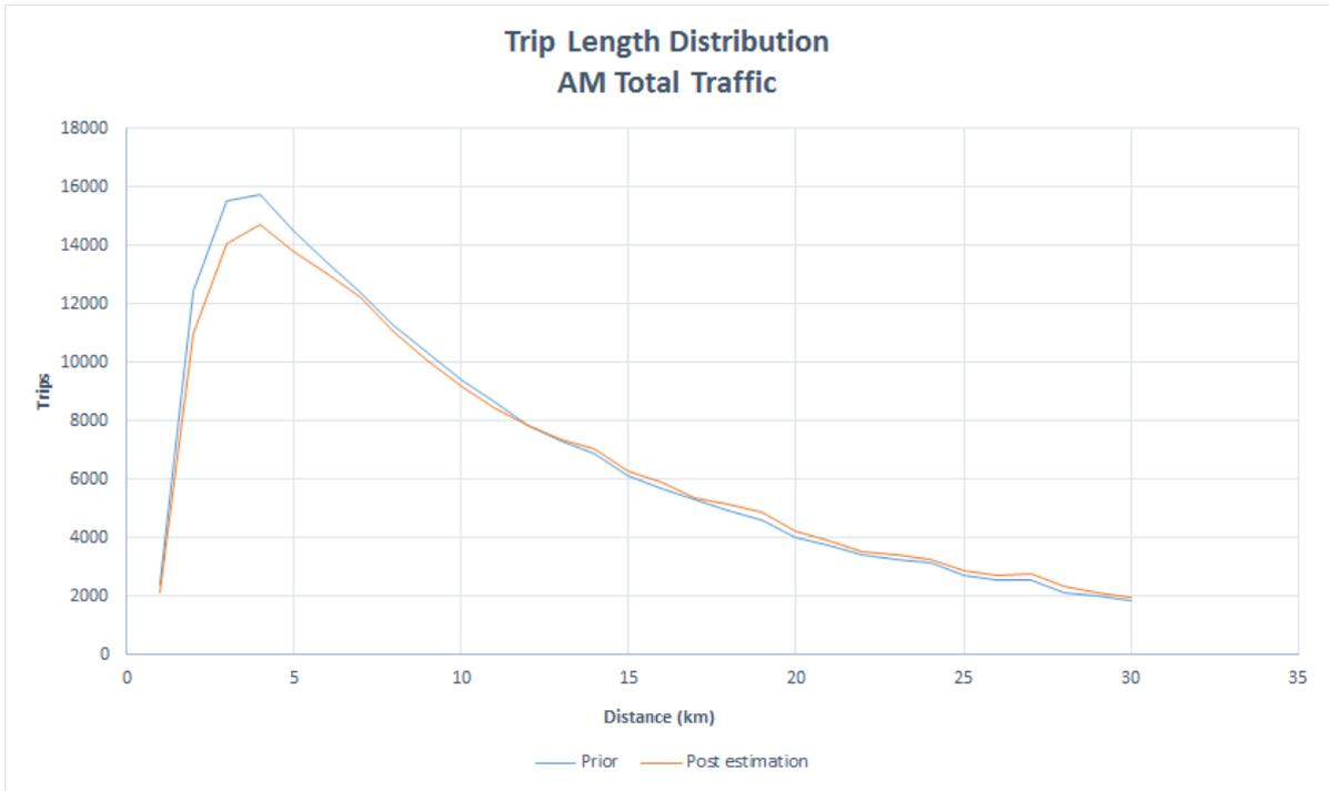
Figure 25. AM Trip Length Distribution for Prior and Post-Matrix Estimation (<30km)
