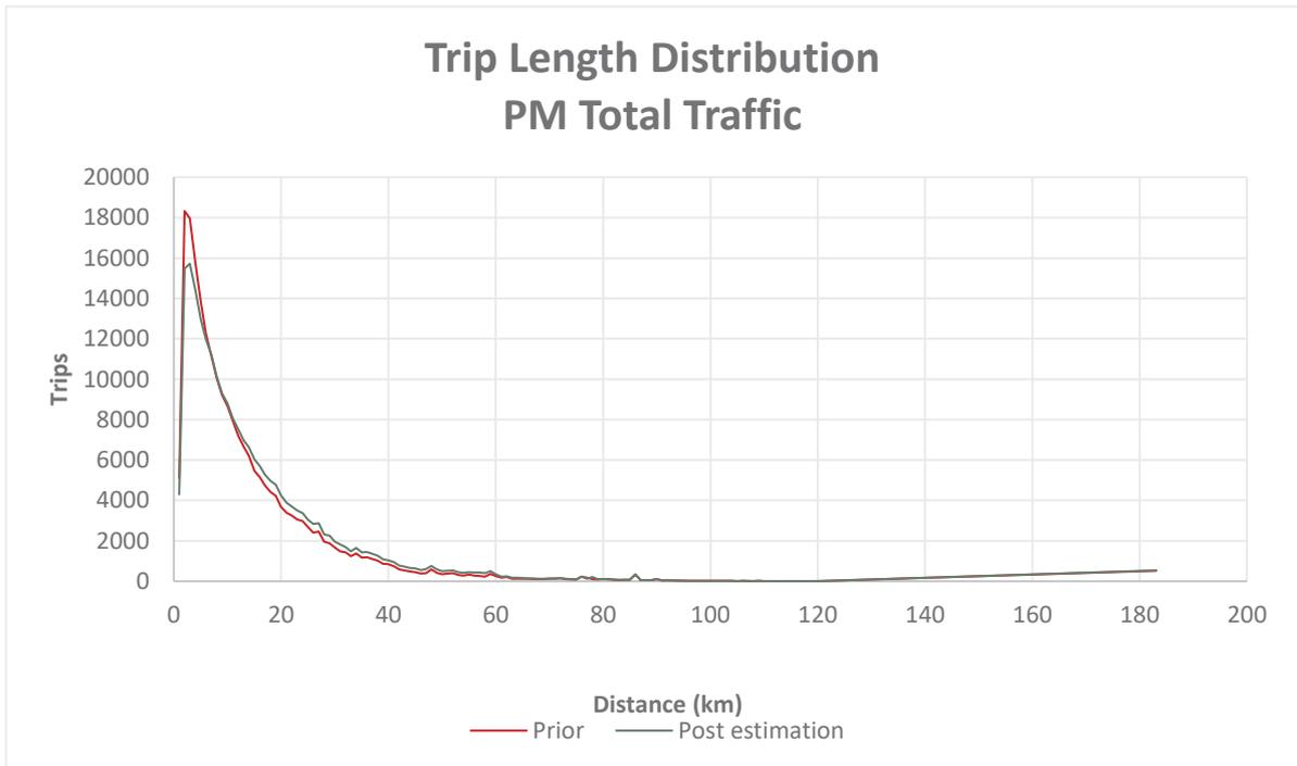
Figure 24. PM Trip Length Distribution for Prior and Post-Matrix Estimation
