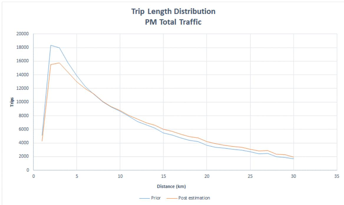
**Figure 27. PM Trip Length Distribution for Prior and Post-Matrix Estimation (<30km)**
