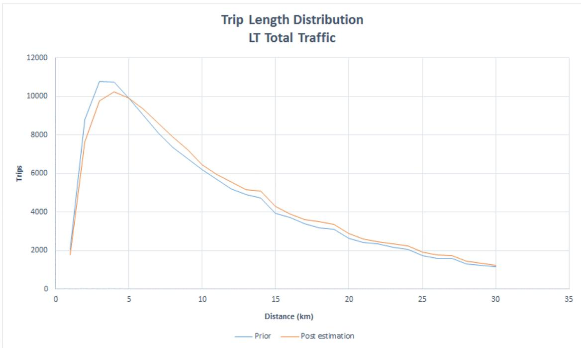
Figure 26. LT Trip Length Distribution for Prior and Post-Matrix Estimation (<30km)
