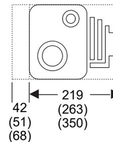
The camera tile is extended on the left by 42 (51) (68) mm (4.5 sw), then the resulting assembly is centred horizontally on the sign.
