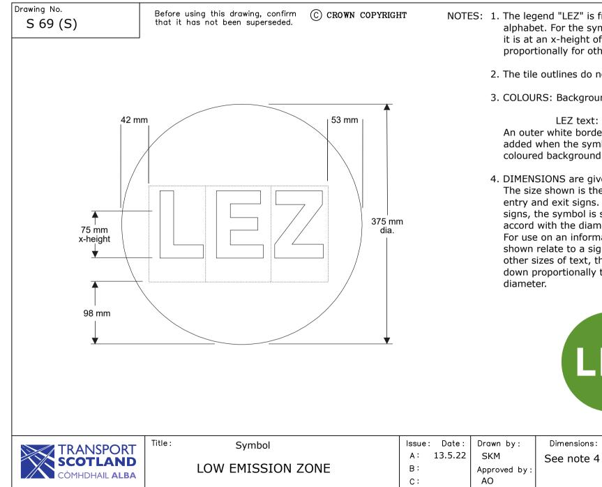
NOTES: 1. The legend "LEZ" is from Transport Heavy alphabet. For the symbol diameter shown, it is at an x-height of 75 mm. This is changed proportionally for other diameters.
