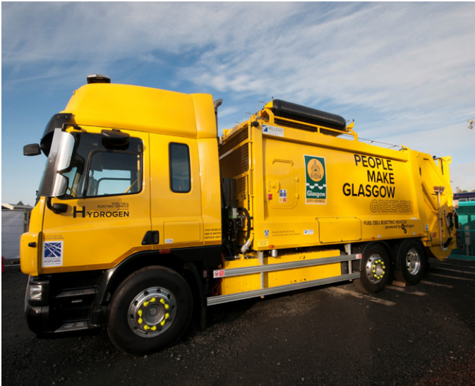
Hydrogen-powered RCV development vehicle for Glasgow City Council.
