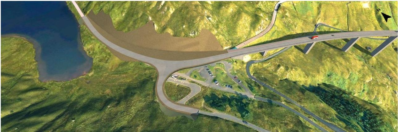
**Figure 3-3 - Visualisation of the B828 junction and associated southbound verge widening for the Yellow Option**
