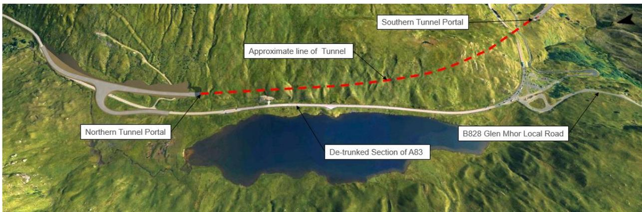
**Figure 3-10 - Visualisation of the Purple Option and the new B828 Glen Mhor local road junction north-east of Loch Restil**
