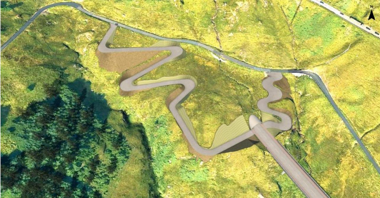
**Figure 5-5 - Construction access from the OMR to the northern abutment / southern portal of the Purple Option**
