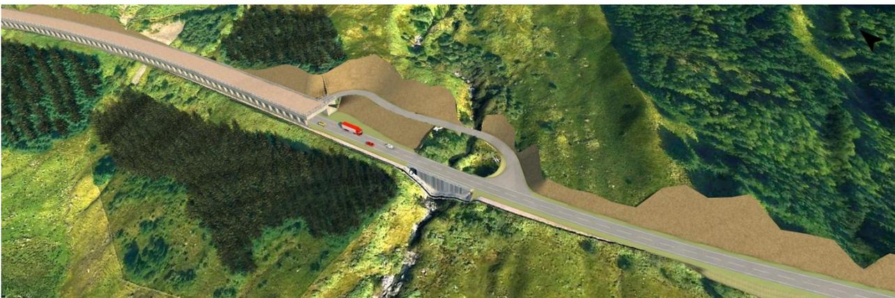
**Figure 5-19 - Visualisation of the maintenance access to the roof of the Debris Flow Shelter for the Brown Option**
