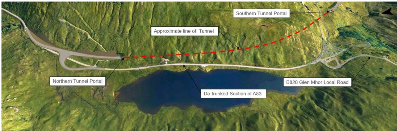
**Figure 5-35 - Visualisation of the proposed B828 Glen Mhor local road junction with the Purple Option to the north-east of Loch Restil**
