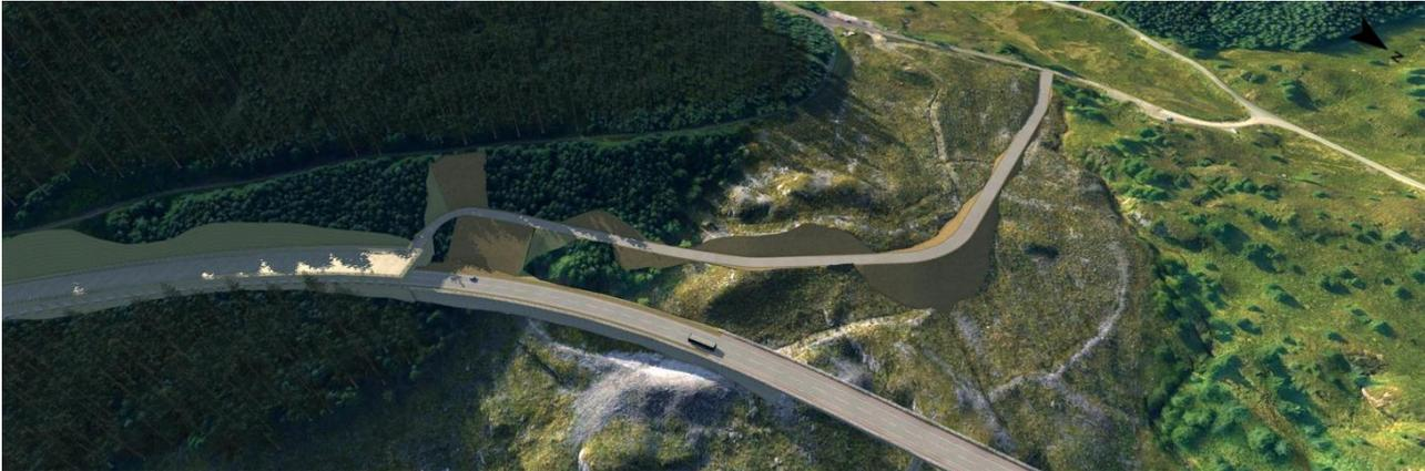
**Figure 5-29 - Visualisation of the northern maintenance access from an existing forestry track that links to the B828 to the roof of the Green Option debris flow shelter**
