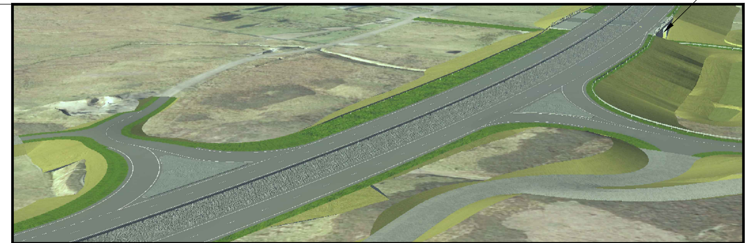
LEFT IN LEFT OFF ON EAST SIDE OF PROPOSED A9(Ch. 25+625)
