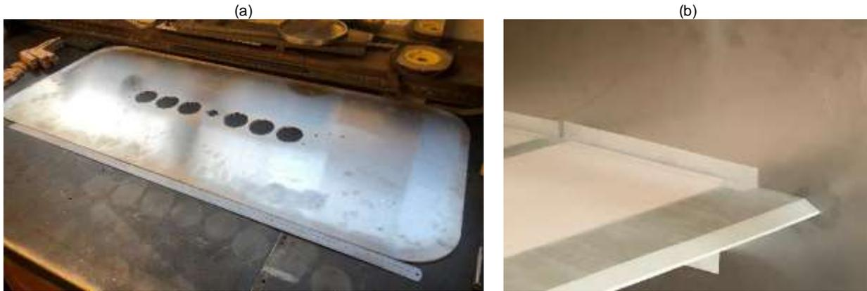
**Figure 2.9.** (a) End plates with holes to access the void of the model; (b) masking tap to seal of gaps between the model and end plates.
