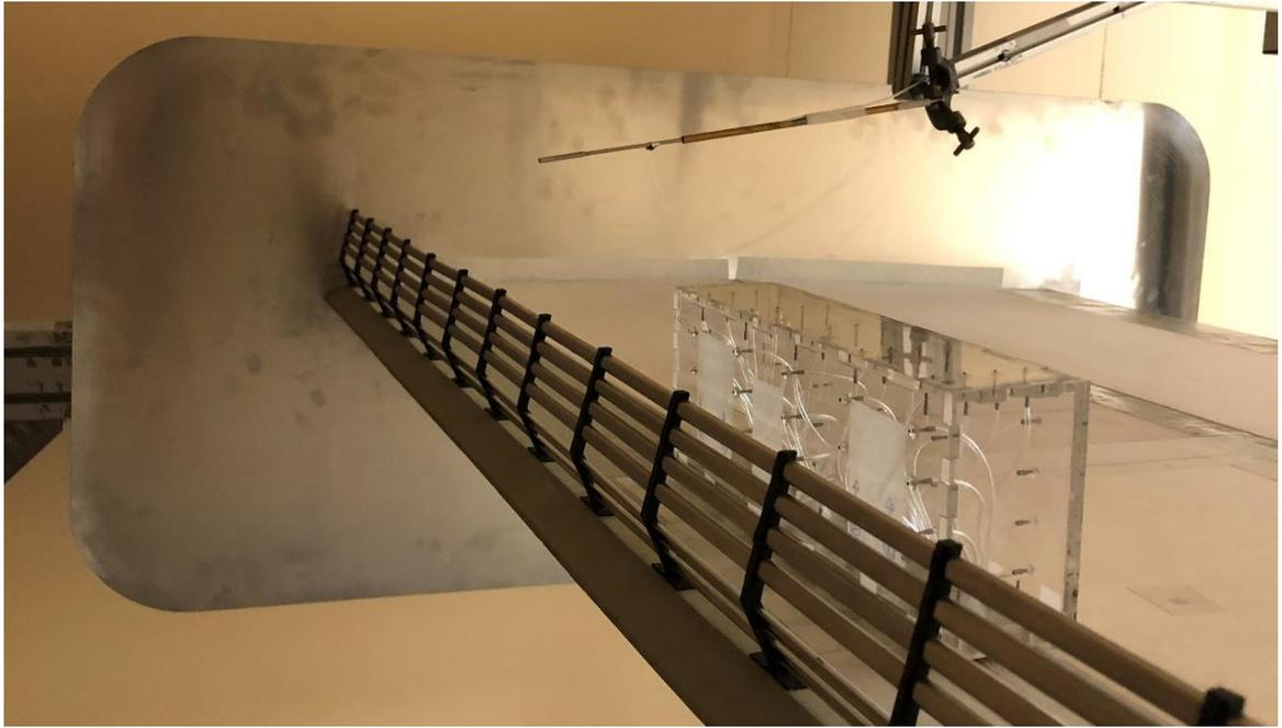
**Figure 20: Wind tunnel model, with carriageway section, wind barrier, and model vehicle located in the hard shoulder (UoN)**
