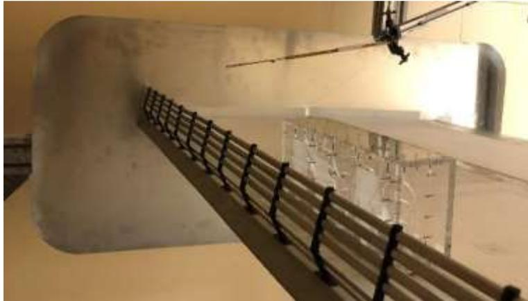
**Figure 2.12.** Wind barrier along the windward edge of the model.
