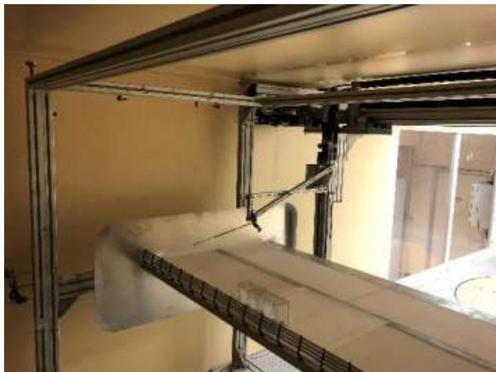
**Figure 2.15.** Wind tunnel sectional model with the wind barrier being attached along the windward edge of the cross section. The reference vehicle is positioned at the centre of the hard shoulder.
