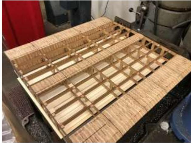
**Figure 2.3.** A complete half of the frame to support the main body of the WT model.
