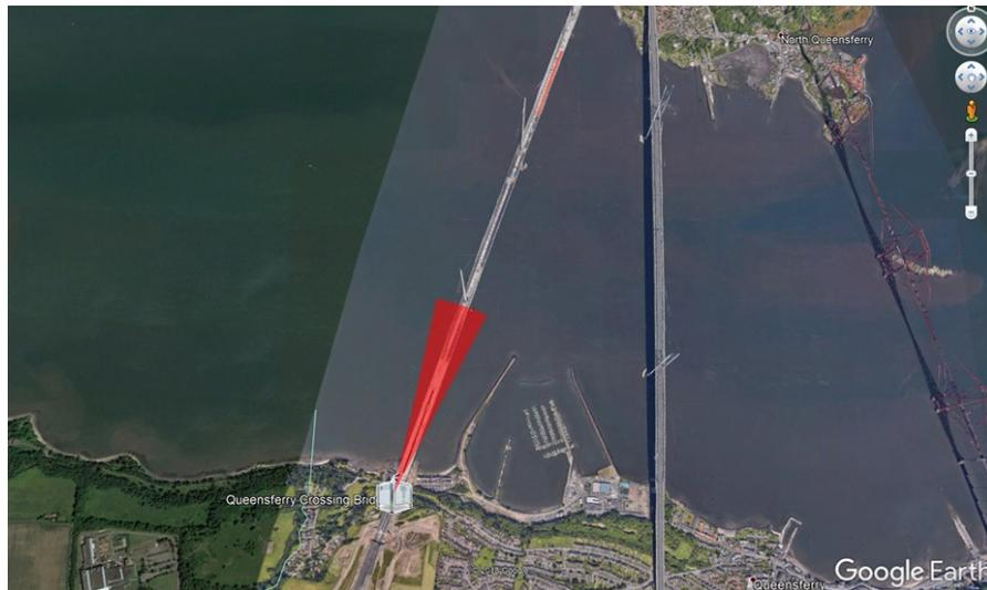
Figure 9 – Scheme of Microscale PPI scan over Queensferry bridge
