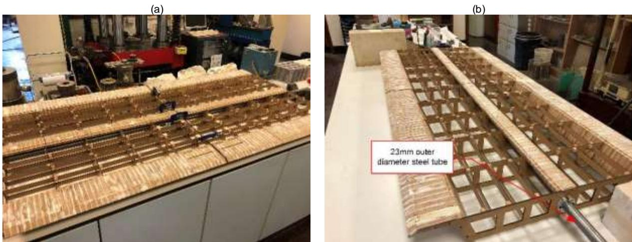
**Figure 2.4.** (a) Two halves of the frame are connected; (b) a 23mm outer diameter steel tube is used as a spine to strengthen the frame.
