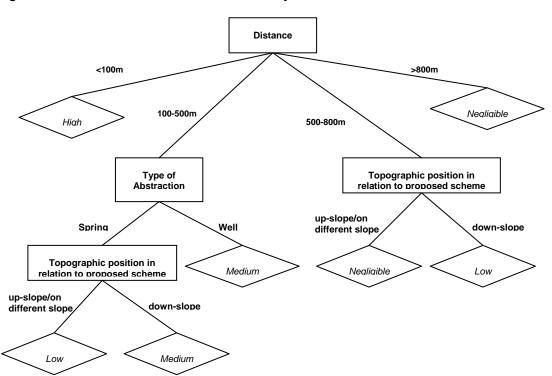
Figure 1: Criteria for the definition of the sensitivity of PWS
